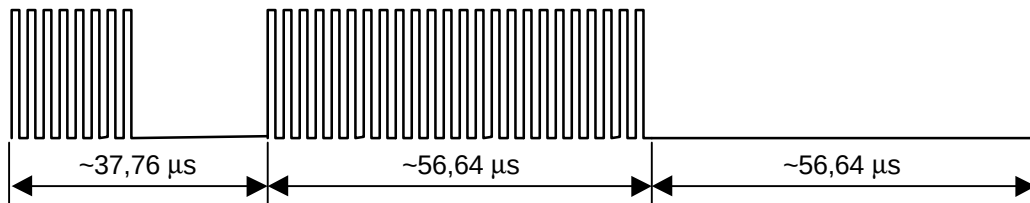
Figure 16 — End of frame when using one subcarrier
