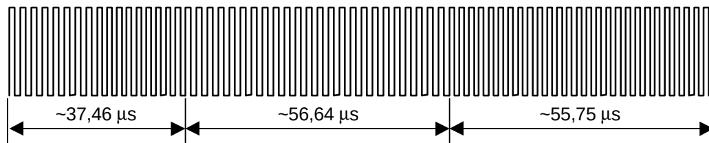
Figure 17 — End of frame when using 2 subcarriers
